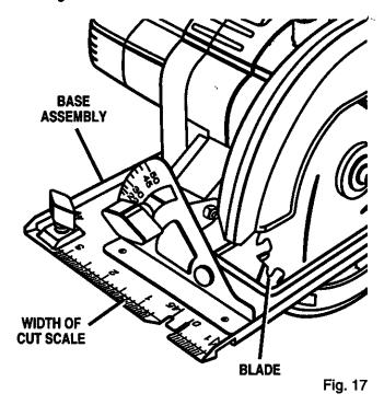
A width of cut scale has been provided on the base of your saw. When making straight cross cuts or rip cuts, the scale can be used to measure up to four inches to the right side of the blade. It can be used to measure up to one inch to the left side of the blade.
